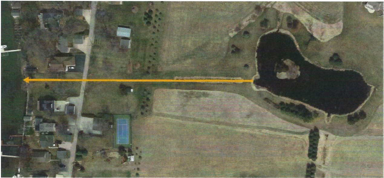
Figure 5 Subbasin 19B Drainage Path and Outlet to Big Cedar Lake
